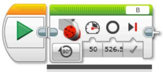
This starts motor B (the left motor if you were facing the same way as the robot) You need to use the sensor readings on your brick to figure out how many degrees in the rotation sensor it takes if you manually turn your robot 90 degrees right. For our robot, this value is 526.5. See the PDF file for more information on how to do this.
