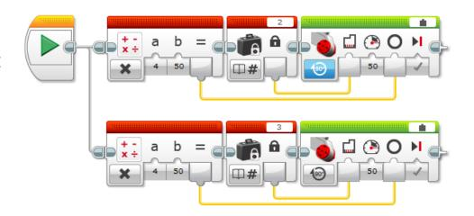
To simplify it, we can make the below My Block (Motor\_Inches) that moves the selected motor forward
