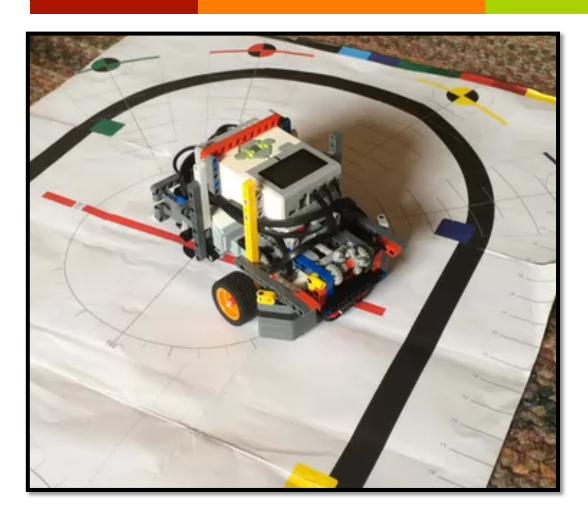
This video shows the robot align to the black line. Even when the robot comes in at a steep angle, it is still able to align well.
