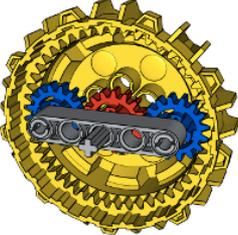
Assuming that the red gear is the input, the gray beam is the output and that the yellow gear is not rotating (e.g. fixed to a motor): specify numbers of teeth for red and yellow gear below, then click calculate.
