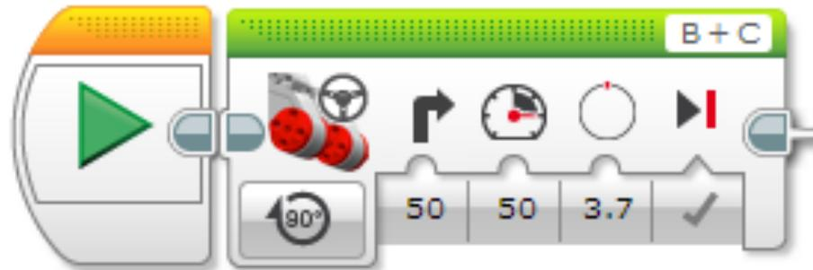
3.7 is the number of motor degrees in 1 protractor degree for Droid Bot. You will have to customize this based on your robot using Step 1A in the Powerpoint instructions.
