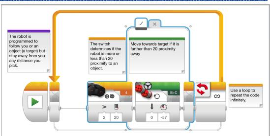
On TRACK3R, the Infrared sensor is BEHIND the robot. Therefore, moving closer to the person is actually moving backwards for the robot! Negative Power = backwards.
